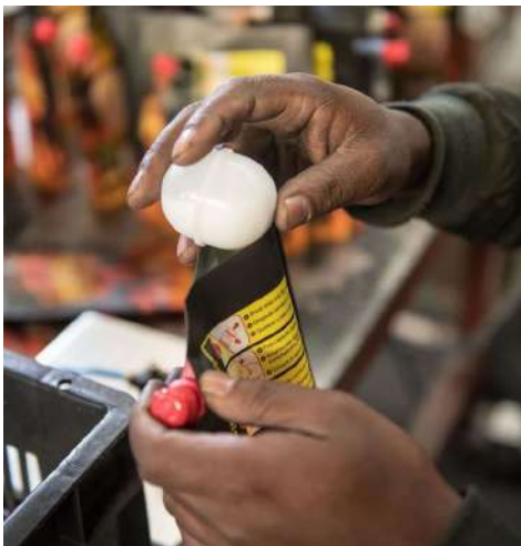
First, the capsule is inserted (left) and then the acetic acid is dispensed into the pouch (right)
