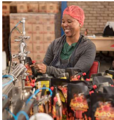
First, the capsule is inserted (left) and then the acetic acid is dispensed into the pouch (right)
